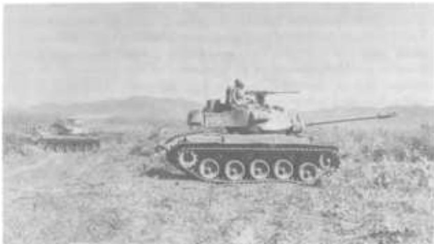
M41 IN SOUTH VIETNAMESE TRAINING OPERATION. Tank has 76-mm. gun, light armor, two machine guns, and crew of four.
