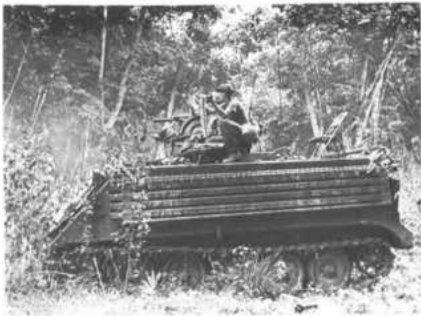
M113 IN ACTION AT BEN CUI RUBBER PLANTATION, AUGUST 1968. Hollow steel planking on sides of vehicle offer protection against shaped charges.
