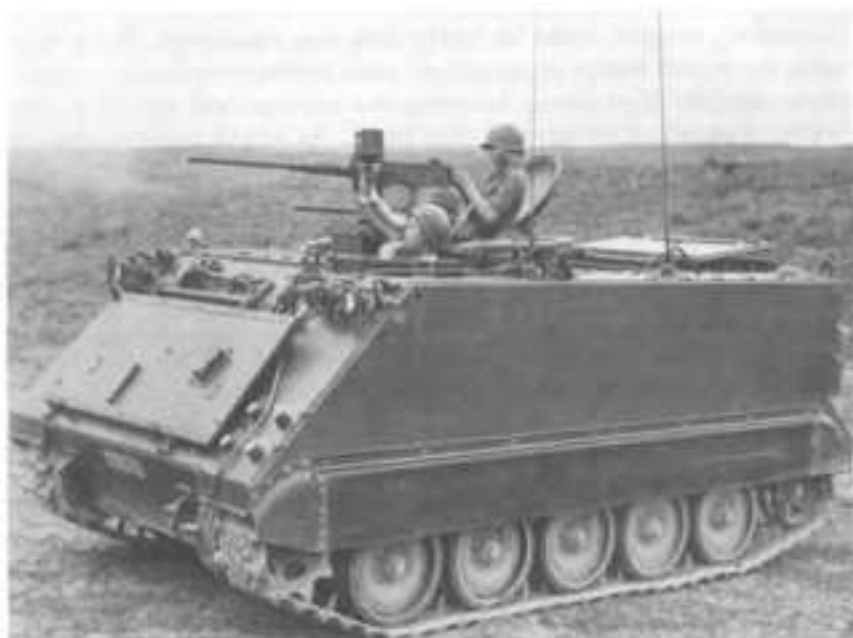
ARMORED PERSONNEL CARRIER, M113, firing .50-caliber machine gun during South Vietnamese training exercise. Barrel of side-mounted .30-caliber machine gun can be seen on far side of M113.
