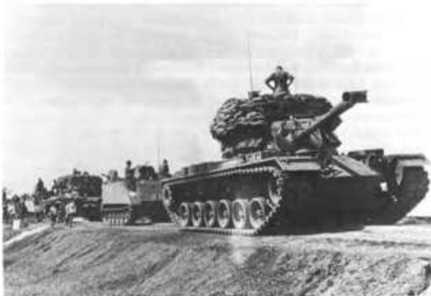
TANKS AND ACAV'S SECURE SUPPLY ROUTES IN 25TH INFANTRY DIVISION AREA. Sandbags modify vehicles for security role as movable pillboxes.
