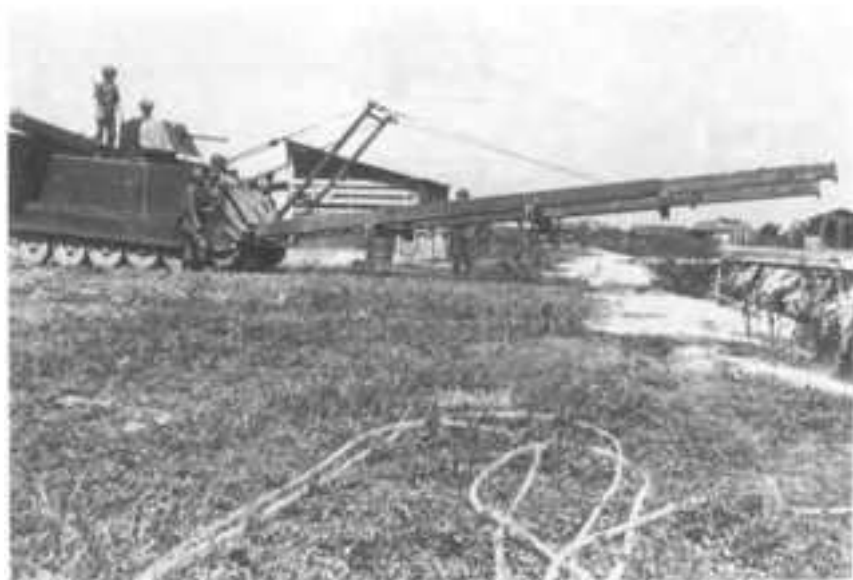
BALK BRIDGE CARRIED BY M113 is demonstrated by troops of South Vietnamese Armor School.
