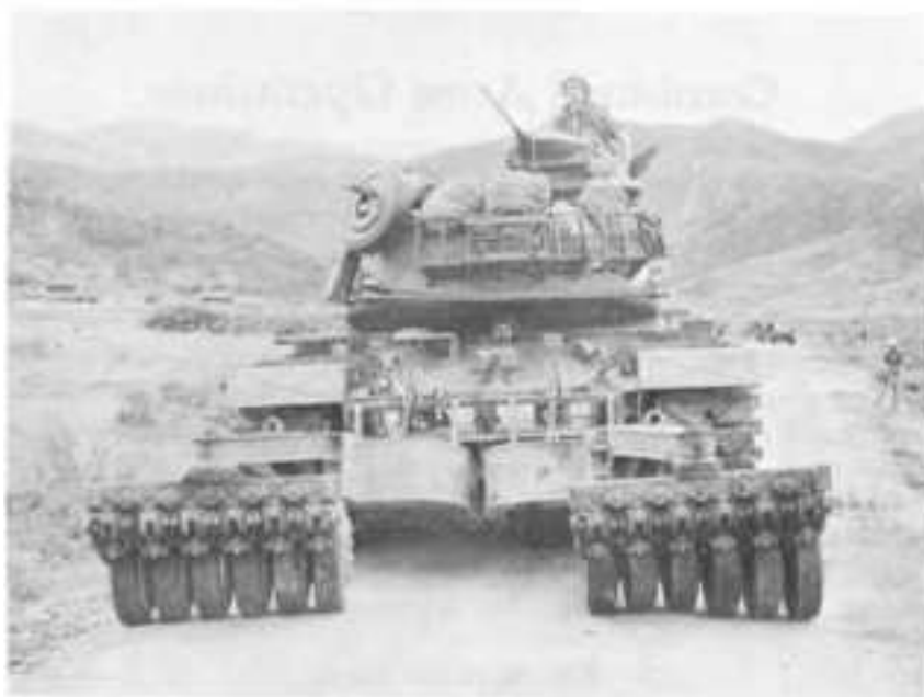
TANK-MOUNTED MINE ROLLER PREPARES TO CLEAR HIGHWAY 19
